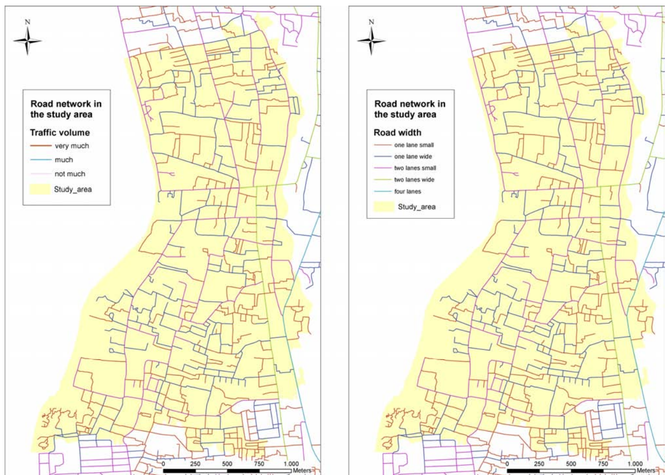
Figure 20 (left) / 21 (right) Traffic volume (left) and road width (right) in the study area (Source: own illustration – Data basis: own data collection; Map basis: Quickbird satellite image)
